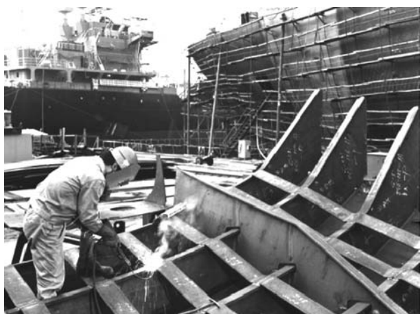
Figure 1: Ilmenite type electrodes shined in shipbuilding throughout the 1960s and 1970s due to excellent usability and weldability.
