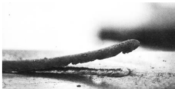
Figure 1: Convenient self-peeling slag removal with RB-26 assures a glossy bead appearance without postweld brushing.
