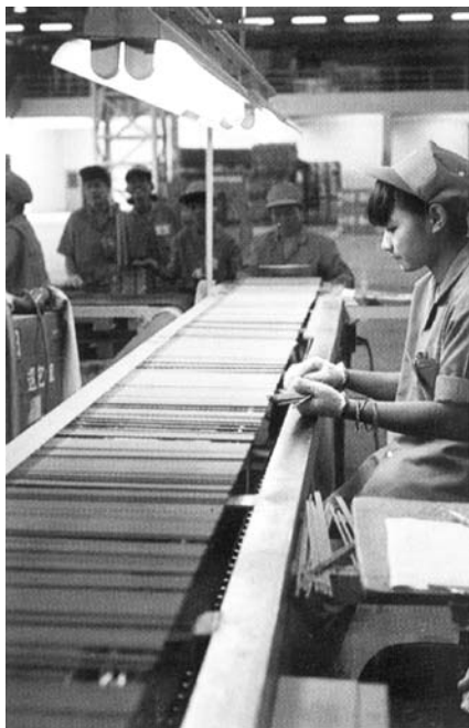
Figure 2: To ensure the appearance quality of RB-26, electrodes are inspected piece by piece in accordance with Kobe Steel's standard (at Thai-Kobe Welding).
