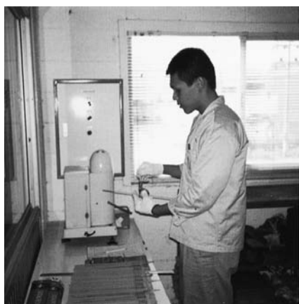
Figure 3: In order to ensure the quality of RB-26, the dimensions of the electrodes are inspected lot by lot by using Kobe Steel's proprietary inspection procedures (at Thai-Kobe Welding).
