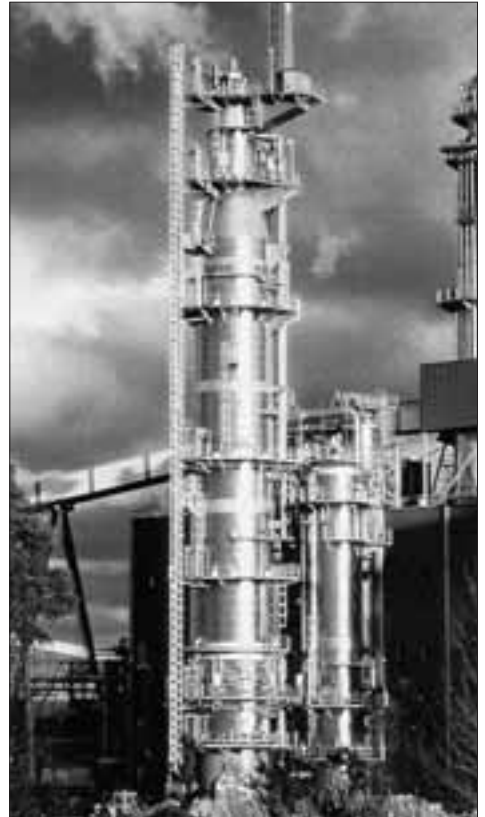
Figure 1.9. High-alloy steels such as 2205 and 254 SMO are widely used in pulp and paper applications
