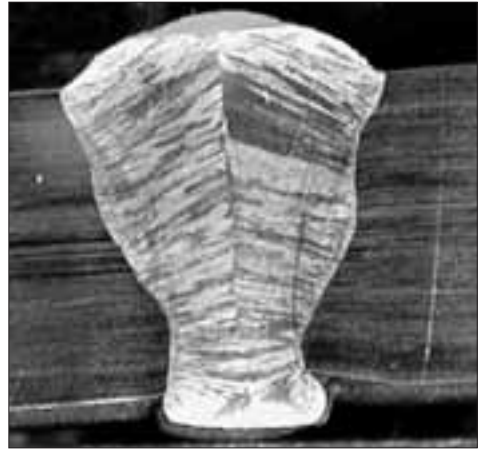
Figure 5.12. Excessive weld metal – MIG 316L-Si
