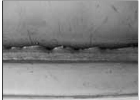
Figure 5.1. Lack of fusion – MIG
